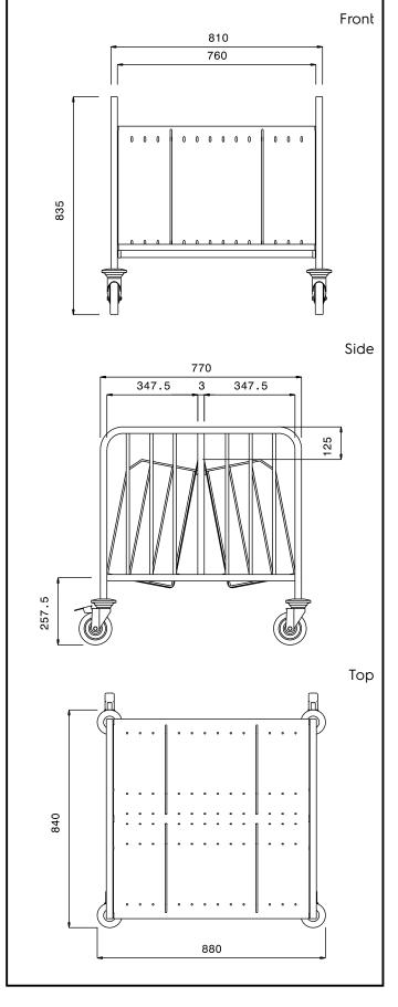
Service Trolleys 2 Side Trolley for 300 plates - height 835 mm
